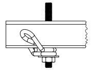
This method is only suitable for use with a 4 way transverse/longitudinal brace. Seismic hooks must be sequenced as shown to align at 45° angle
